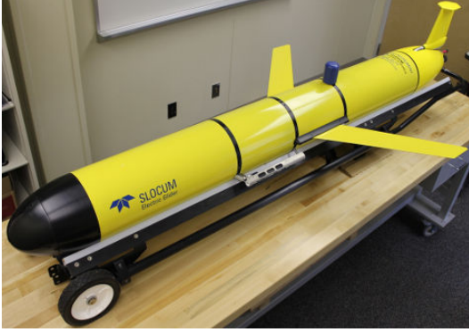
Figure 1: A Slocum Glider equipped with a double payload bay and an acoustic modem.
