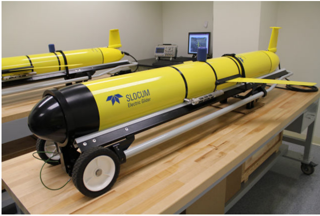
Fig. 3. Two Slocum Electric Gliders equipped with WHOI acoustic Micro-Modems. The modem's transducer is the protruding cylinder on one of the science bays.
