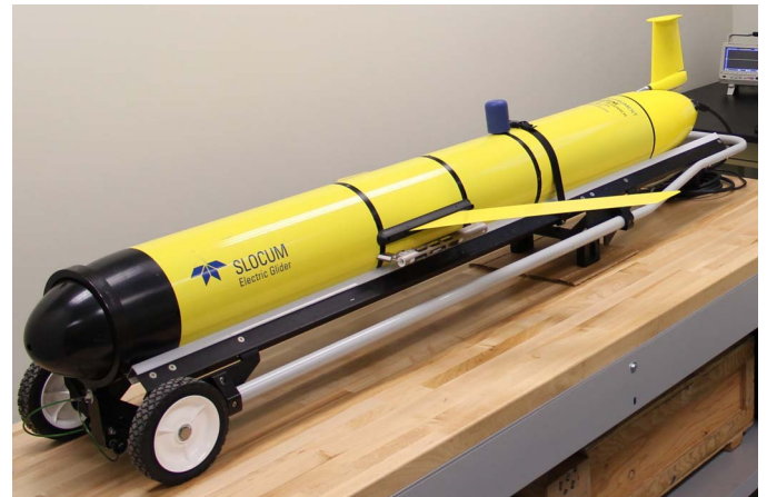
Fig. 1. A Slocum Glider with a double payload bay and a top-mounted acoustic modem in its deployment cart.
