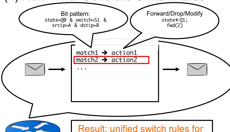
Result: unified switch rules for forwarding and measurement
