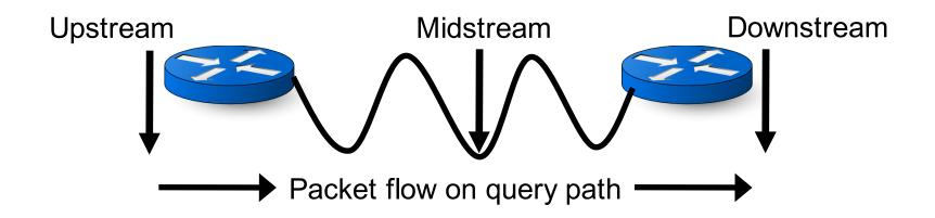
Match predicates at switch ingress, egress or both in\_atom(dstip=128.1.2.3) in\_out\_atom(dstip=128.1.2.3, dstip=10.1.2.3)
