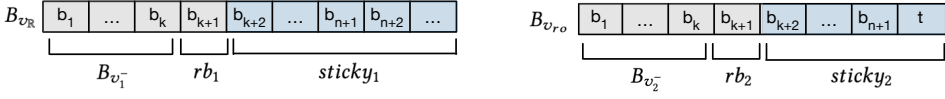
Fig. 12. Rounding components while rounding v_{\mathbb{R}} and v_{r_o} to \mathbb{T}_k . We show the bit-string of v_{\mathbb{R}} in extended infinite precision representation. Note v_{r_o} is a value in \mathbb{T}_{n+2} .
