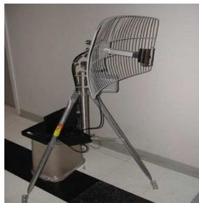
Fig. 1. Our rotating directional antenna landmark.
