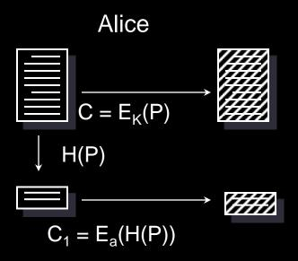
Alice picks a random key, *K*, and encrypts the message (P) with it using a symmetric algorithm.
