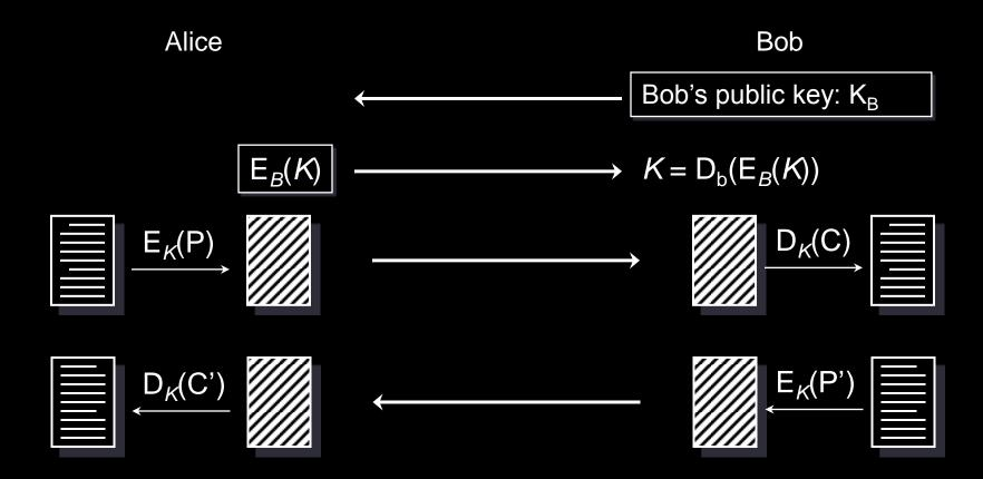
decrypt message using a symmetric algorithm and key *K*
