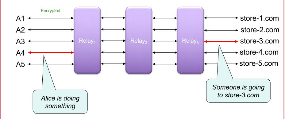
Tor uses (by default) three layers of relays.
