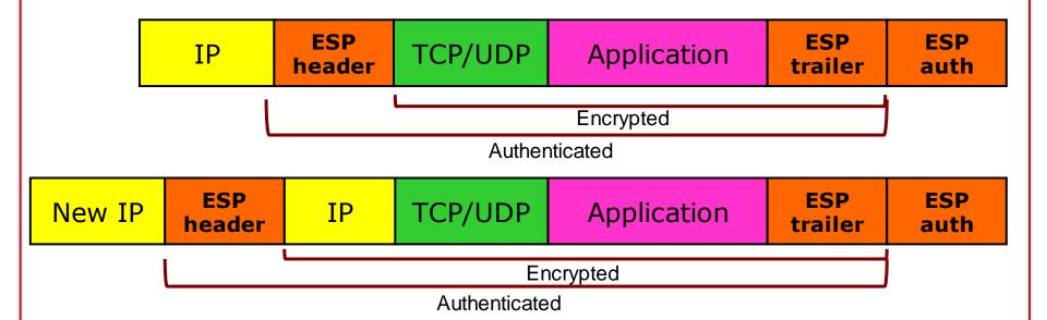
Directly on top of IP (protocol 51) - not UDP or TCP
