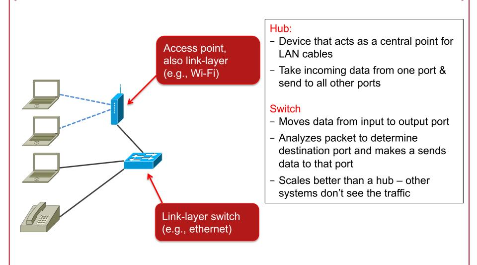
Link-layer switches: create a physical network (e.g., Ethernet, Wi-Fi)
