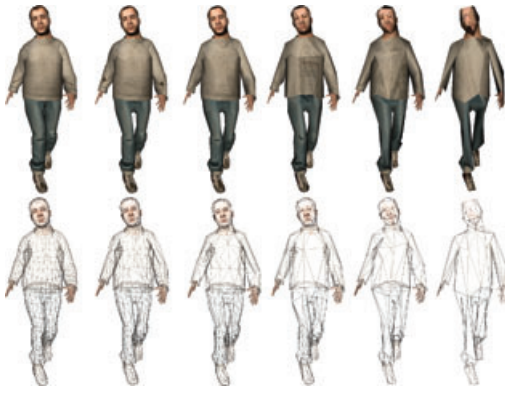
Figure 10: From left to right we show the original mesh M_{100} and some examples of the simplified meshes M_{75} , M_{55} , M_{35} , M_{20} and M_{2.5} .
