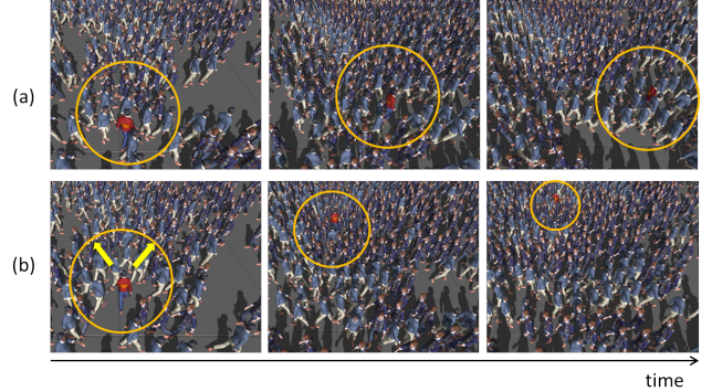
Figure 7: Pushing through dense crowd: The red agent pushes through a dense crowd that moves perpendicular to its direction of travel. Agents are simulated using (a) anticipatory collision avoidance only, and (b) combination of anticipatory collision avoidance and physically-based interaction. In the latter case, the red agent can proceed to its goals quickly by pushing other agents through its path.
