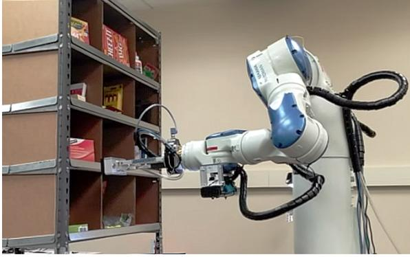
Fig. 3. The data collection setup for the warehouse pick-and-place dataset: A Motoman SDA10F robot and an Amazon-Kiva Pod stocked with objects. At this configuration, the Kinect sensor mounted on the arm is used to detect an object at the bottom row of shelf bins.
