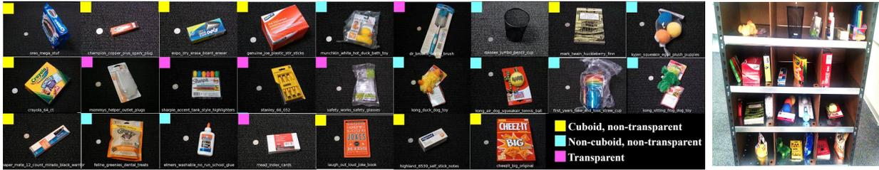
Fig. 2. (Left) Items used in the Amazon Picking Challenge 2015 and featured in the dataset. Three groups of objects are identified based on their effects on pose estimation from RGB-D data: a) cuboid and non-transparent, b) non-cuboid and non-transparent, c) transparent. (Right) An arrangement of the shelf with the APC objects.
