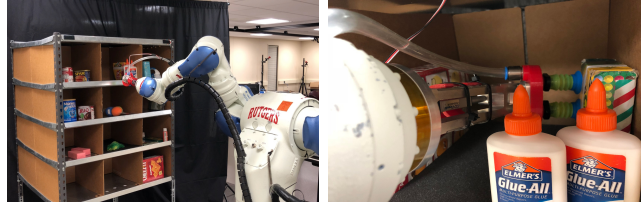
Fig. 1. An example of manipulation in cluttered table and shelf environments, where the grasped object is partially occluded by other objects.
