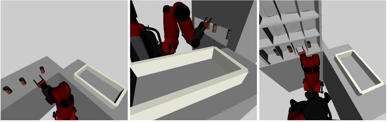
Fig. 5. The three versions of the environment for evaluating the methods, inspired by the Amazon Picking Challenge. From left to right: easy, medium, hard. The offline roadmaps are computed given the easy environment. This problem involves a Baxter arm grasping an object from the tabletop in a vertical configuration and placing it inside a box in a horizontal configuration. The medium challenge has the objects placed inside a shelf that was not known during the construction of the roadmap and which limits the motion of the robot. The hard challenge has multiple shelves, the objects placed deeper inside these shelves, which further limits the capability of the arm of grasping these items.
