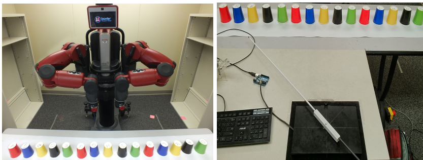
Fig. 3. (left) The start position of the trajectories on the Baxter robot during the experimental setup. (right) A view of the pointing device from the subject's perspective.
