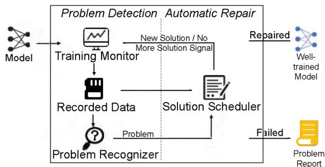
Figure 2. Overarching Design of AUTOTRAINER
