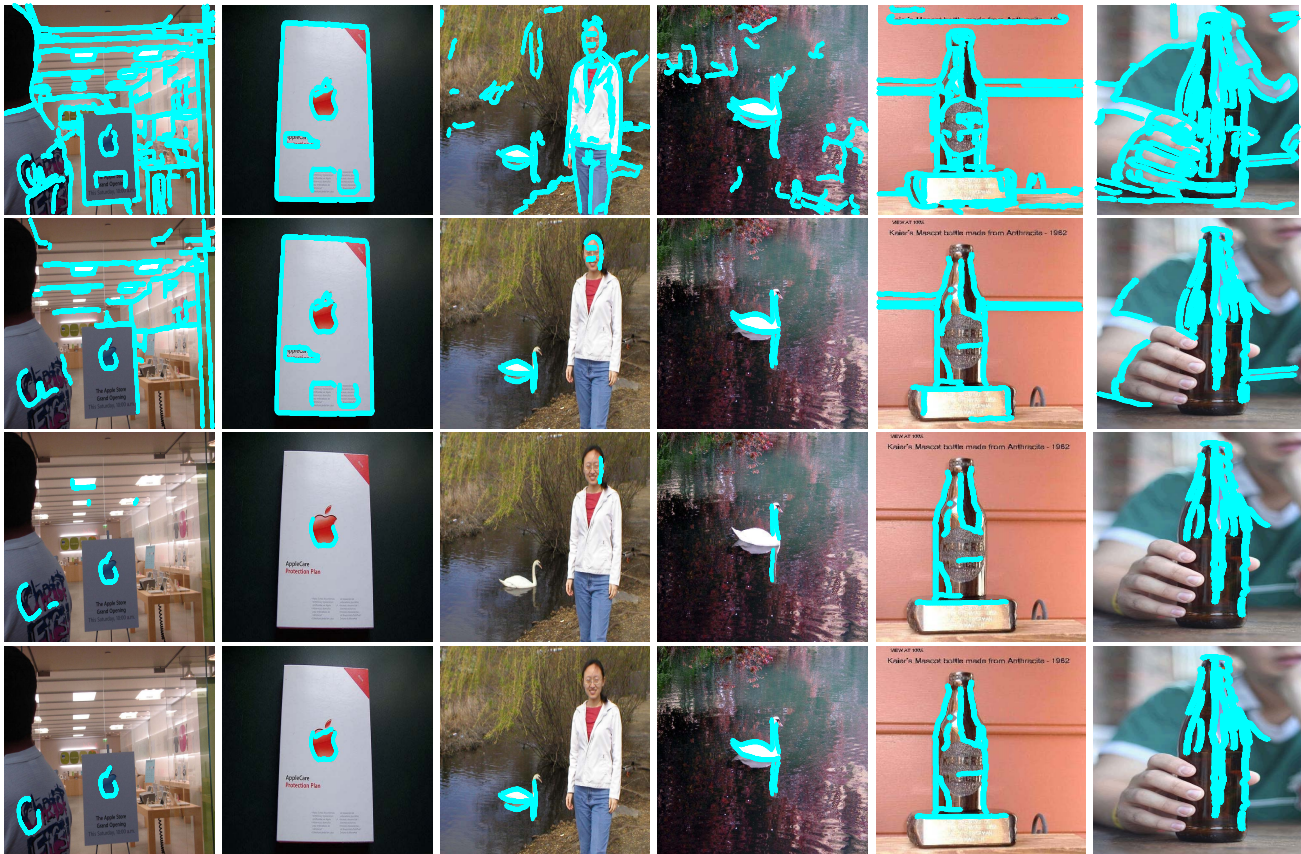
Figure 4. Qualitative performances of proposed method for detecting edges on objects (from left to right) apple logos, swan and bottle. Rows: top to bottom, input edges, edges with p(\text{KAS} \in \text{object}) > p(\text{KAS} \in \text{bckgnd}) , proposed linear, proposed nonlinear.
