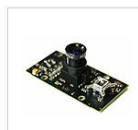
USB-powered single board PMD camera
