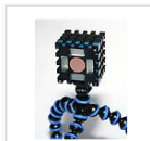
USB-powered TOF camera out of the European ARTTS project
