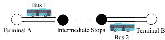
Fig. 16. Existing bus operating and charging patterns.
