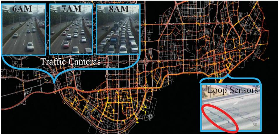
Fig. 10. Loop detectors and traffic cameras.
