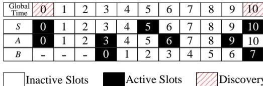
**Figure 1. Neighbor Discovery Process.** Device  $S$ ,  $A$ , and  $B$  start their local timers at global time 0, 0, and 3, respectively. According to Disco,  $S$  will discover device  $A$  and  $B$  at global slots 0 and 10, respectively, based on their duty cycles, i.e., 20% ( $\frac{1}{5}$ ), 33% ( $\frac{1}{3}$ ), and 14% ( $\frac{1}{7}$ ).
